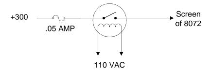
The bias line that is normally controlled by K1 must be shorted (Short A5-259 to A10-5). According to Amperite, there is no problem controlling 300 VDC since heater to ground spec is 800 VDC.
